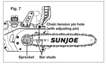
7. Adjust the chain tension as needed by adjusting the chain tensioner screw with the supplied flat-tip blade screwdriver. Make sure to align the chain tensioner screw with the pin hole (Fig. 8).
