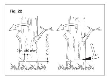
Make the lower horizontal notching cut first.
