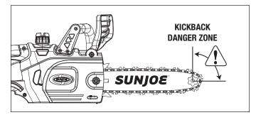
⚠WARNING! Kickback may occur when the nose or tip of the guide bar touches an object, or when the wood closes in and pinches the saw chain in the cut.
