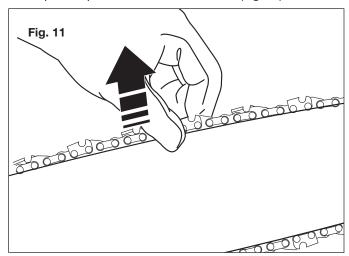
Loosen the brake by pressing both the switch and the safety button. Using a screwdriver, run the chain along the guides to check that it moves smoothly.
