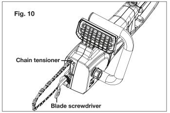
2. The tension is correct when the drive links on the chain do not slip out of the chain guide on the bar when the chain is pulled up from the middle of the bar (Fig. 11).
